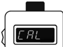
3. With the **blo** message on the display, press the **access button** on the side of the BAT **once** to enter calibration mode (**CAL**).
