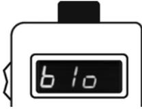
3. With the **blo** message on the display, instruct the test subject to blow moderately and continuously into the mouthpiece. A constant tone indicates the breath sample is being properly provided and - - - - is on the display.
