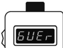
3. With the **blo** message on the display, press the **access button** on the side of the BAT **four times** to enter gas calibration mode (**GVEr**).
