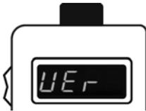
3. With the **blo** message on the display, press the **access button** on the side of the BAT **three times** to enter calibration mode (**VEr**).
