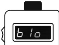
9. Wait for **blo** to appear on the display. Press and hold the valve down to release the gas.
