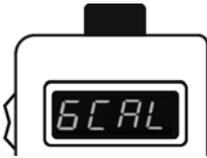
5. With the **blo** message on the display, press the **access button** on the side of the BAT **twice** to enter gas calibration mode (**GCAL**).
