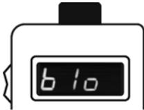
7. Wait for **blo** to appear on the display. Turn the air source on. A tone sounds and - - - is displayed indicating proper air flow.
