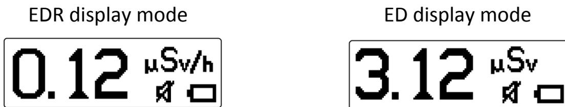
Figure 11 – The dosimeter display in EDR, “Search” and ED display modes, briefly;
