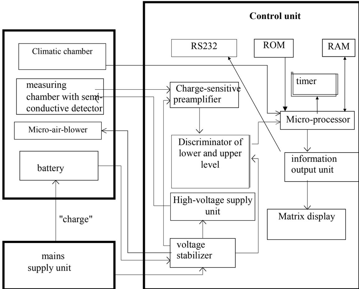
Figure 2. Functional diagram of the radiometer.
