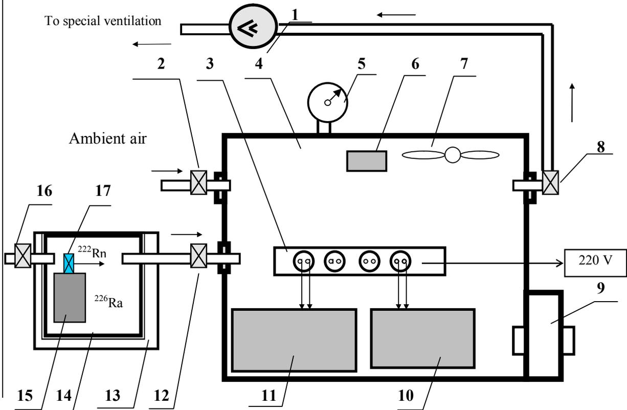
Figure 4. Diagram for verification of the radiometer
